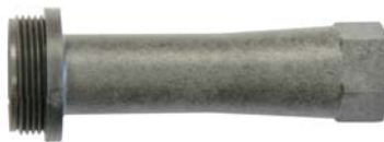
venturi 25882A485 I.D. .470", tapers to .620"
