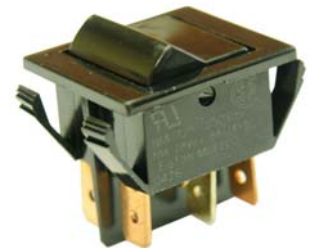
DPDT on-off-on rocker switch 16A 125/250 VAC / 10A 28VDC 6 terminals, ref. # 260411E approximate base size: 7/8 x 7/8
