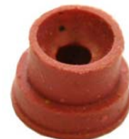
grease fitting covers, bright red molded rubber, internal lip holds cap in place & keeps paint, cleaning fluid & dirt out
