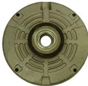
5.5" TE drive endbell brg size : 6203 c/w 2-1/4 rubber mount
