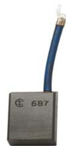
3/8 x 1 x 1-1/2 long, graphite shunt : 2" long + 3/16" "U" terminal, top & bottom bevel
