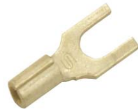
open terminal 16-14 wire size, 0.281" stud size
