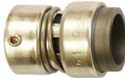
rotary for old style VMS pumps 14mm shaft size, silicon carbide face uncompressed length : 30mm fastened on shaft with set screw
