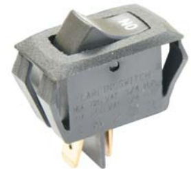
SPST on-off rocker switch 3/4hp 16A 125VAC 3/4hp 10A 250VAC, 2 terminals approx. base size : 1/2 x 15/16
